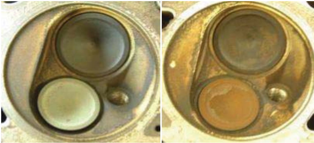
Figure 2. Cylinder heads (intake is black and exhaust is greenish or reddish) from one of the dissected Ford Escorts. After 100,000 miles of use, reddish Manganese deposits can be seen on the MMT exhaust valve of the cylinder head (right). [3, 7, 8].
