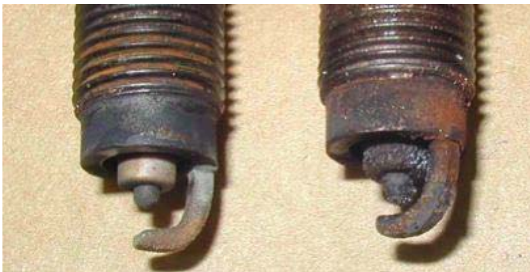
Figure 1. Digital photos of the clear-fuel (Left) and MMT spark plug (right) [3, 7, 8].
