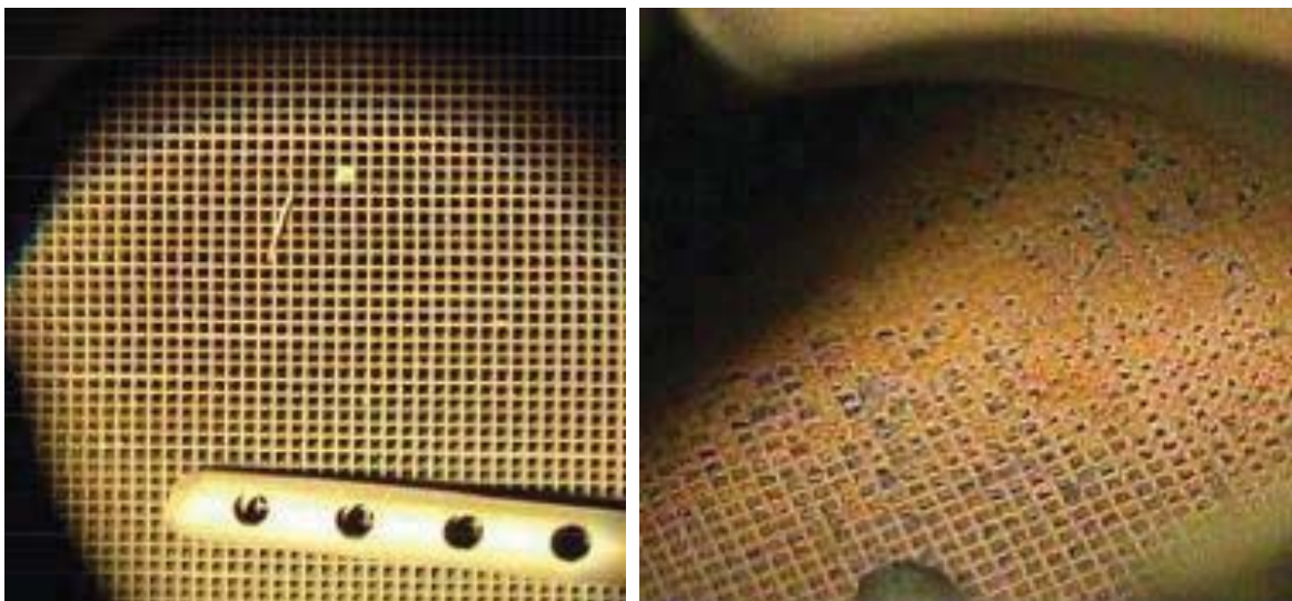
Figure 3. Digital photos of the clear-fuel and MMT catalyst at the end of the test program. The photo of the MMT-catalyst (right) shows that 20% of the cells are blocked. [3, 7, 8].
